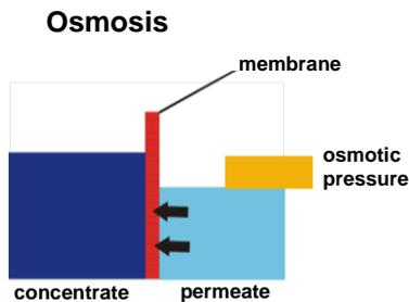
If the sequence is reversed by applying pressure on the higher concentrated solution, clear water penetrates the membrane in reverse direction after the osmotic pressure has been overcome. Dissolved salt is retained. Such process is called reverse osmosis.
