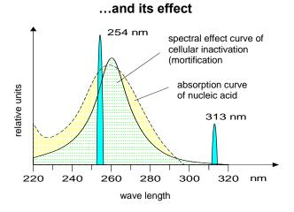
The efficiency of UV systems is determined by the light transmission of the water.
